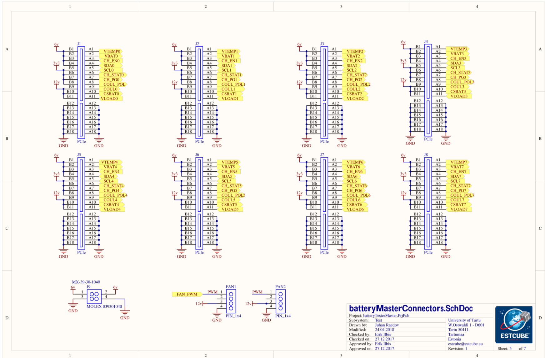
Figure 18. Main board connectors schematics
