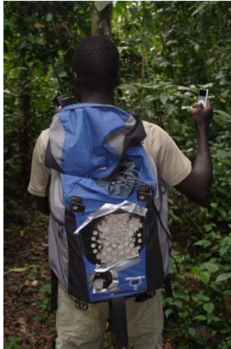
Figure 6.1: Photograph illustrating the speaker used to conduct playbacks, concealed in a rucksack.
