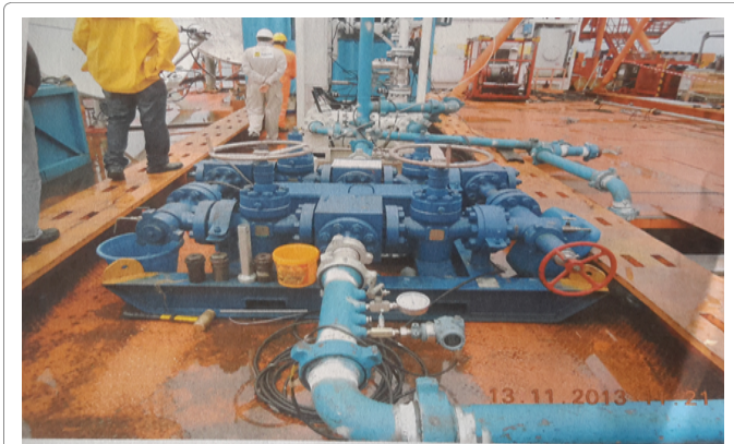
Figure 1: Typical choke manifold with adjustable and fixed choke boxes for multi-rate well test.
