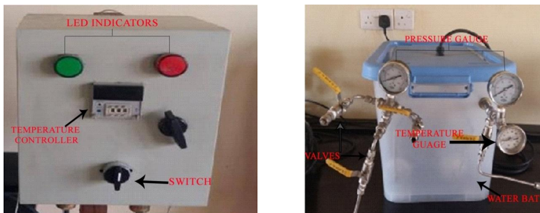
Fig. 2. Fabricated sorption isotherm equipment for Nigerian coal
