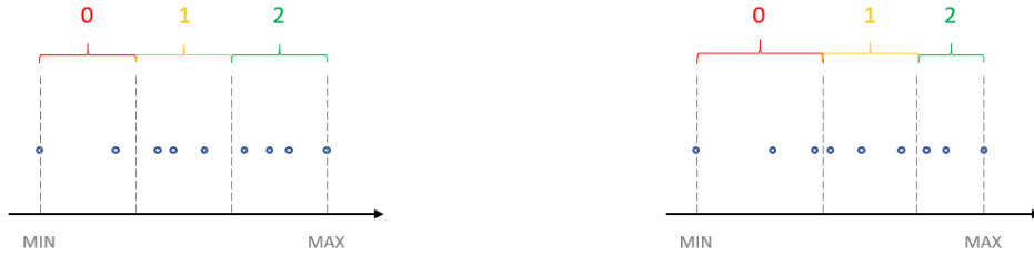
Figure 11. Comparison between the adaptive threshold method (left) and the quantile threshold method (right).
