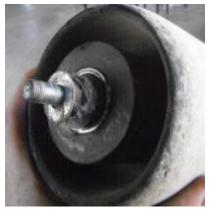
2.2a Review failure item - axle bearing's obstruction to rolling
