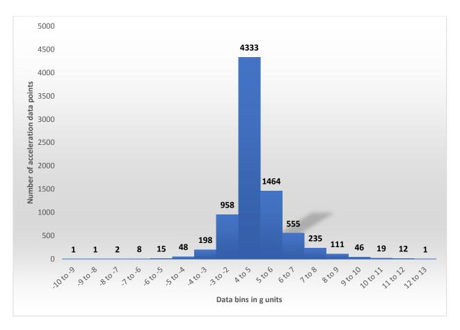
Figure 22. Accelerations seen by the HKC caster in the field (User 1)
