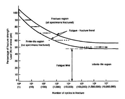
Figure E 3. Fatigue curve for typical medium strength steels[142]
