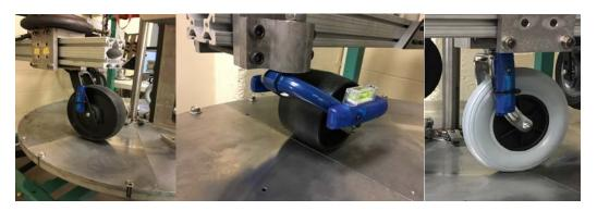
Figure 19. Accelerometers installed on MRT (left), WRR (center) and HKC (right) casters
