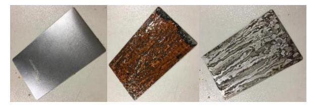
Figure 26. Mass loss test panel before corrosion (left), corroded panel after 100hrs of salt fog exposure (center) and cleaned panel before weighing (right)
