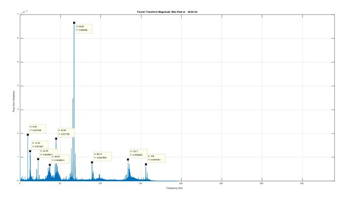
Figure D 1. FFT for vibrations seen on caster arm in forward direction
