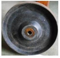
2.1a Review failure item - axle bearing corrosion
