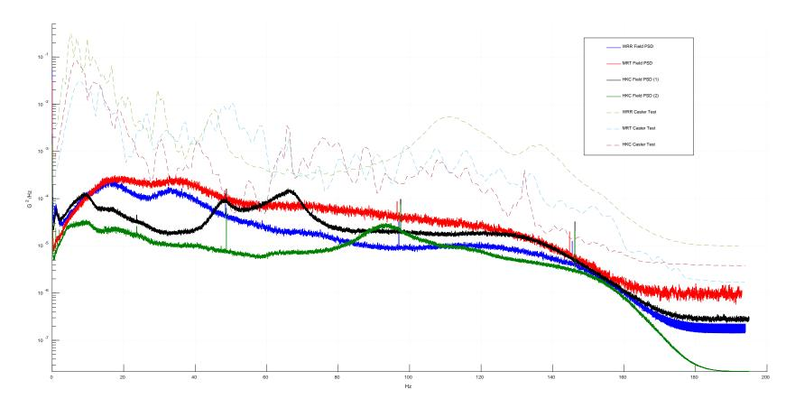
Figure 20. PSDs of accelerations seen by caster models and their wheelchair frames in the field
