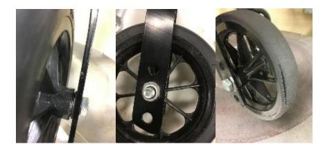
Figure 36. Model D failures. Shock tested samples (left and center) and abrasion + shock tested sample (right)
