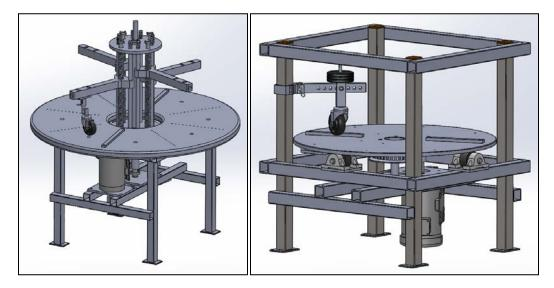
Figure B 2. Caster assembly test design concepts #4 (left) and #5 (right)
