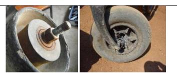
Corroded caster bearing from an ISO tested wheelchair after 15 months of use (left) and fractured bearing (right)
