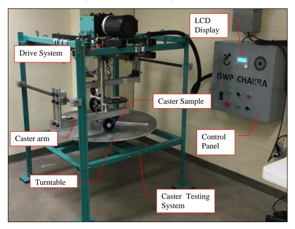
Figure 9. ISWP Caster Assembly Test
