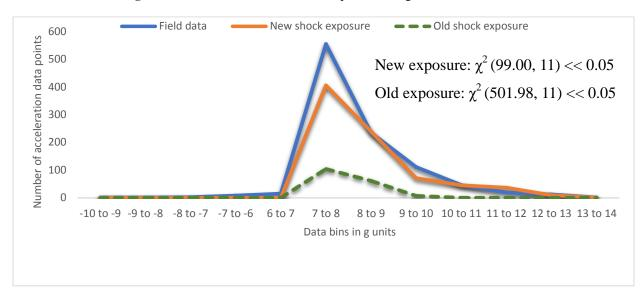
Figure 24. Field and caster test shock exposure histograms for WRR caster
