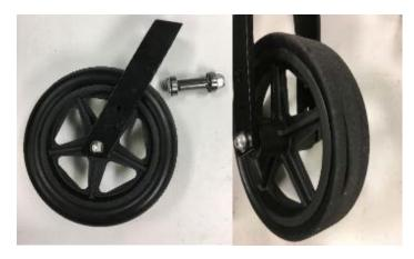
Figure 37. Model E failures. Shock tested sample (left) and abrasion + shock tested sample (right)
