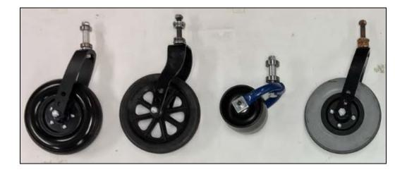
Figure 10. Caster assemblies tested in initial testing phase (Models A-D from left to right)
