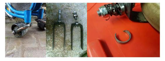
Figure 16. Caster failures with Whirlwind Roughrider (left), Sunrise Quickie Rumba (center) and Invacare
