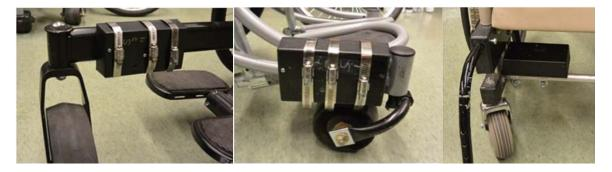
Figure 18. Accelerometers on MRT (left), WRR (center) and HKC (right) wheelchairs
