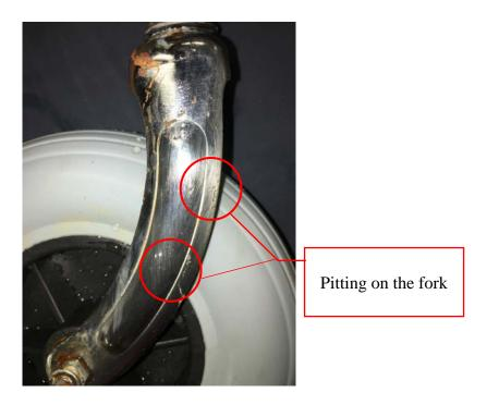
Figure 38. Corrosion effects on a chrome plated caster fork
