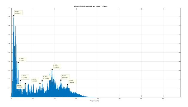
Figure D 9. FFT for vibrations seen on Whirlwind Roughrider caster fork in vertical direction
