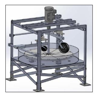
Figure B 3. Turntable design concept
