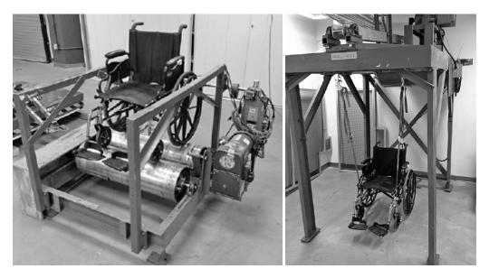
Figure A 1. MDT (left) and CDT (right) without test dummies [74]
