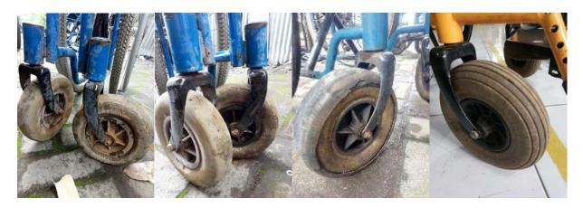
Figure 15. Caster failures with Harmony wheelchairs.
