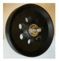
3. Bicycle axle and bearing set (spoke flanges removed)
