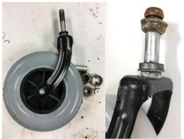
Figure 44. Failure mode seen with model G, bearing fractures (left) and fork crack (right)
