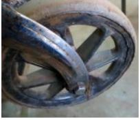
Failure Mode: Etching or Cracking
