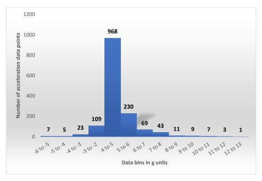
Figure 23. Accelerations seen by the HKC caster in the field (User 2)
