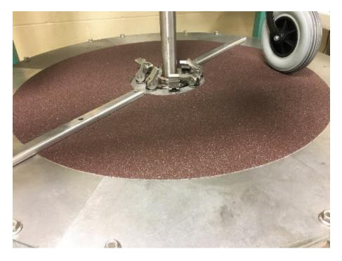
Figure 27. Sanding disc attached to the turntable to simulate abrasion
