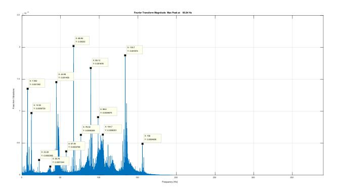
Figure D 2. FFT for vibrations seen on caster arm in lateral direction
