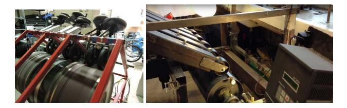
Figure B 1. Caster testing drum equipment with wheelchair manufacturers
