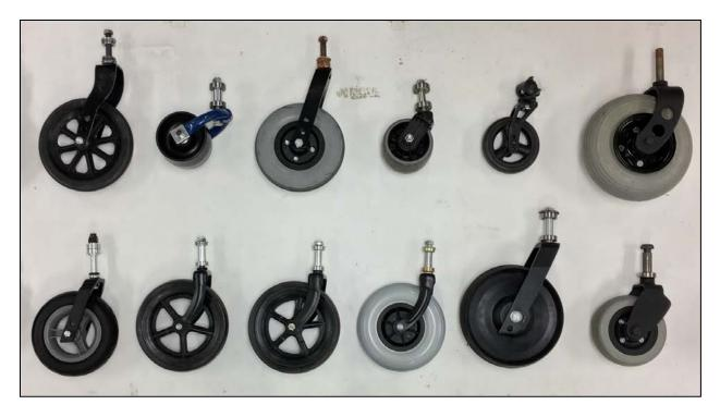
Figure 5. Caster designs used on wheelchairs
