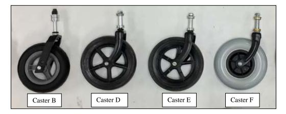
Figure 11. Caster assemblies tested in preliminary testing study (Model A and C are not shown)
