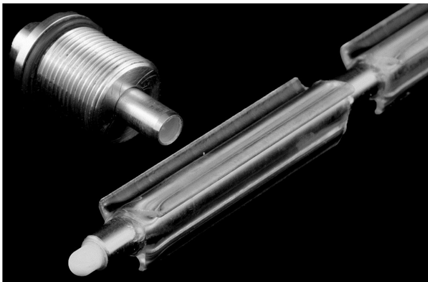
Figure 5.3. Distal end of ULFED driveshaft showing impellers and bearings. Impellers/bearings from Device 3 – (4 cm length, 11.7 mm diameter), ceramic pivot bearing, and UHMWPE bearing cup.
