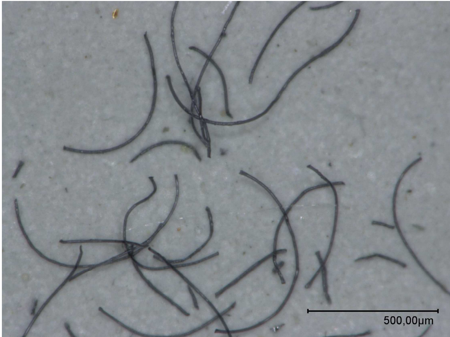
Figure S3: Close up image of the 100% PES fibers released from the textiles after washing.
