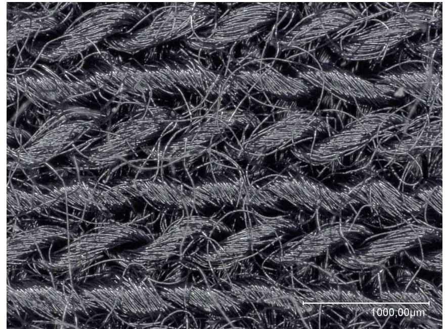
Figure S1: Close up images of the 100% PES interlock and jersey knit variants, where structural differences of the textile are clear
