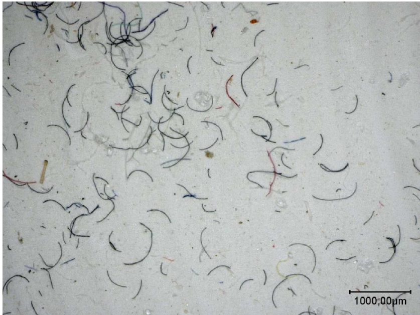
Figure S2: Snapshot of a typical filter image for textiles which have not undergone a pre-wash step (left figure) and which have had a prewash step before the experimental procedure (right figure). Without a pre-wash, it is evident that fibers and residues of different colors and morphologies have collected on the fabric during exposure to air and are subsequently released during the pre-wash cycle in DI water for 5 minutes. When fabrics undergo a pre-wash step before the experiment, only black fibers are present, which are consistent with the test textile at hand.
