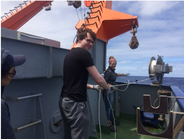
Deployment of free-falling microstructure profiler with a tethered rope for recovery.
