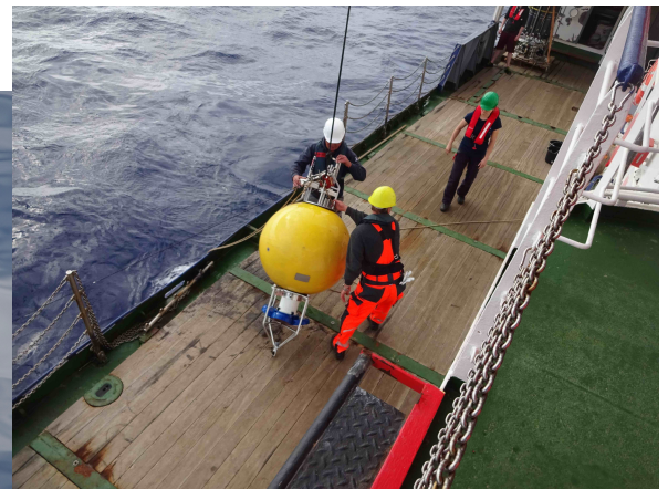
The head buoy housing a current profiler is the first part of the mooring to be recovered after 9 months in the ocean. Photo: T. Reitz
