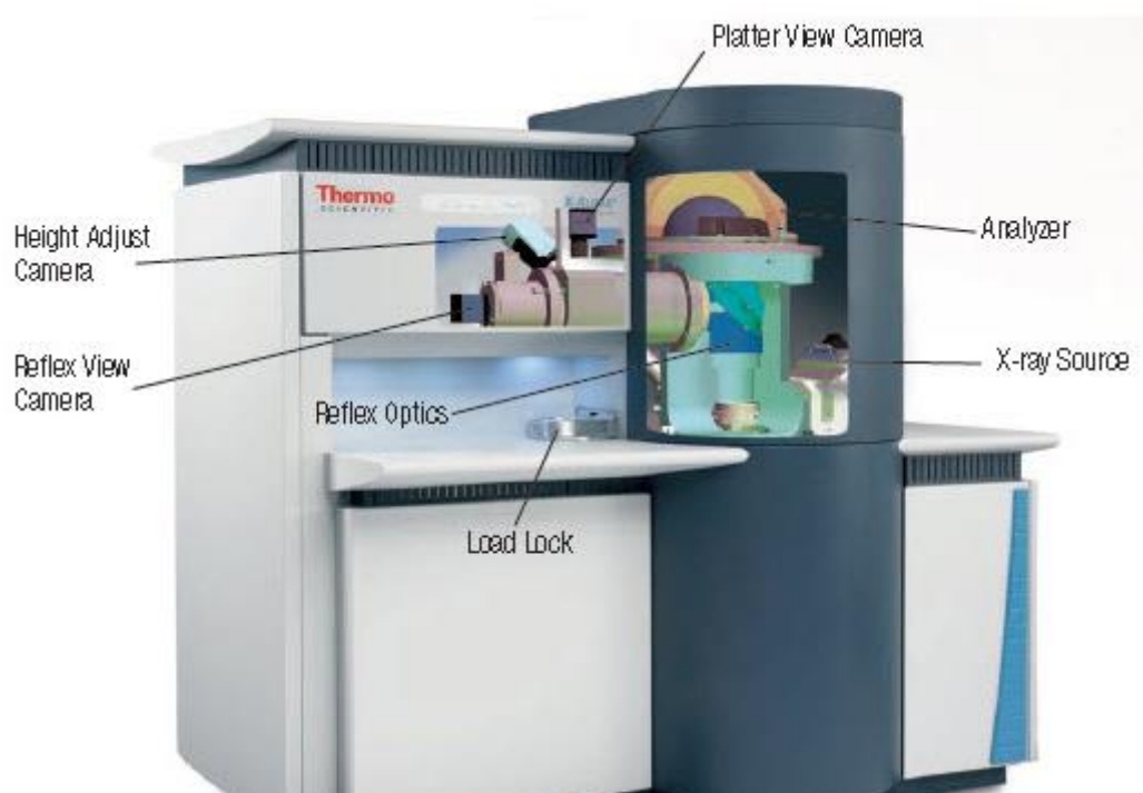
Figure 10. The ThermoScientific K-Alpha XPS apparatus (image provided by the vender's site).
