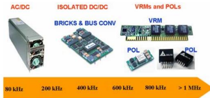
Figure 1.2: Switching frequency of different voltage regulators [1]
