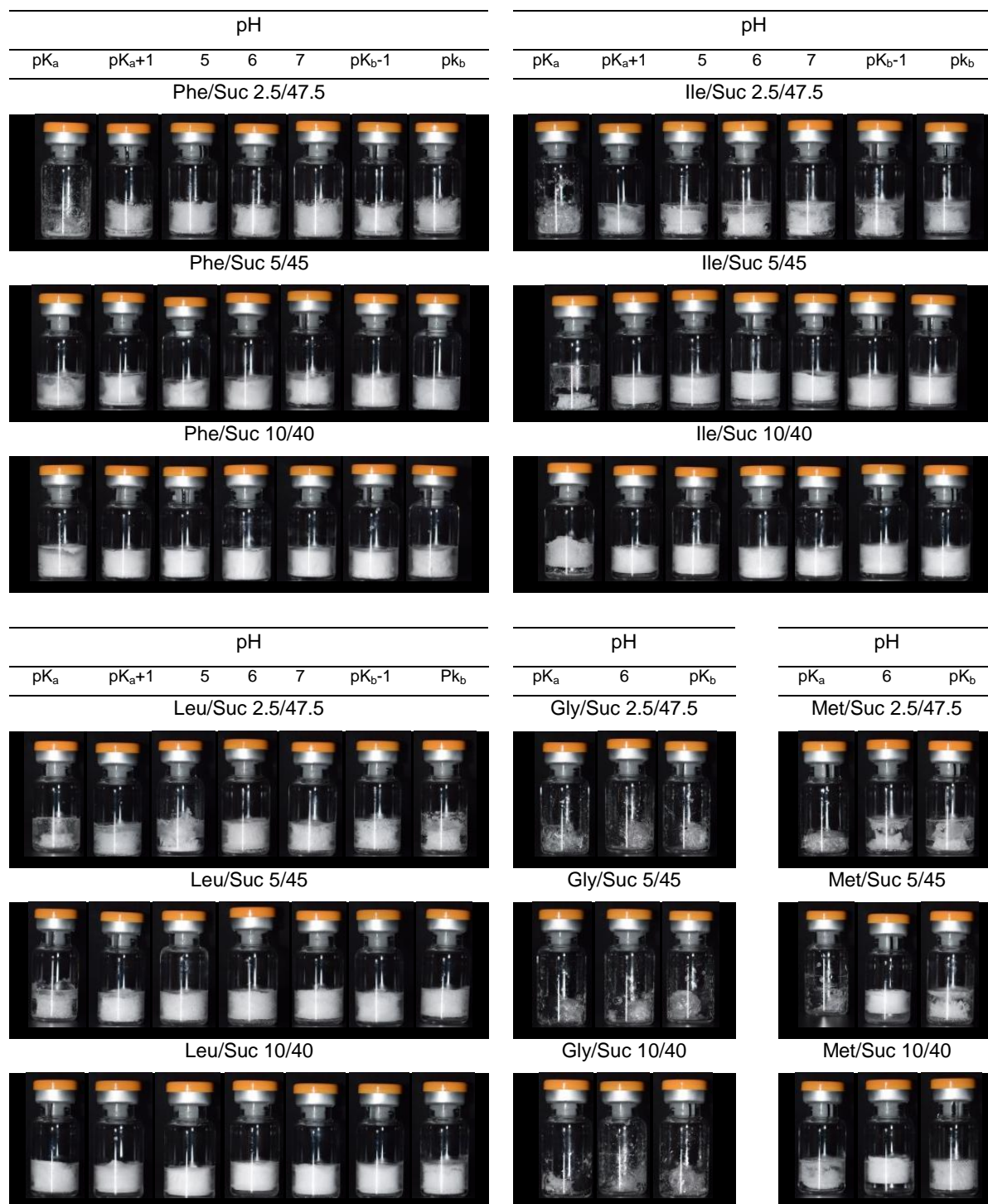
Figure 8-5. Macroscopic Appearance of AA/Suc lyophilizates at different formulation pH freeze-dried without annealing step (Table 6-3).
