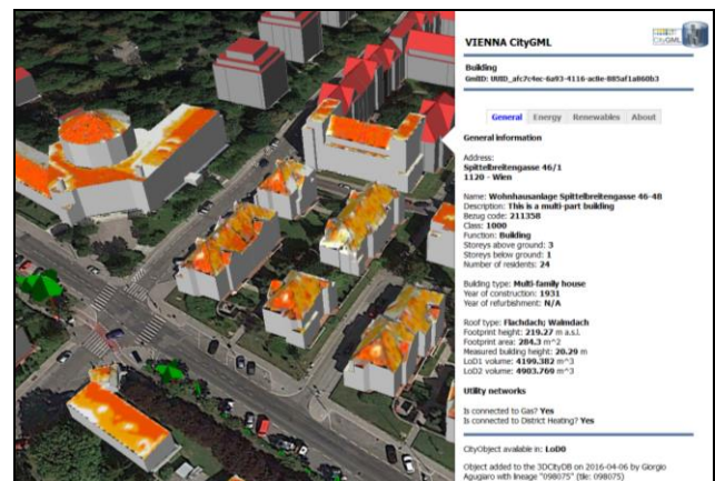
Figure 2. Example of visualisation of the 3D city model in Google Earth; thematic data for each building can be accessed in the balloon
