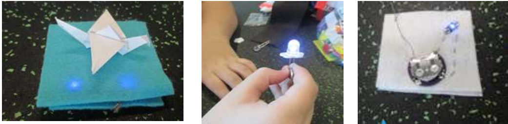
Figure 2.3 Emma's projects (from left to right): The swan swimming in a lake, an LED inserted into a flower-shaped button, the e-textile base for her corsage.
