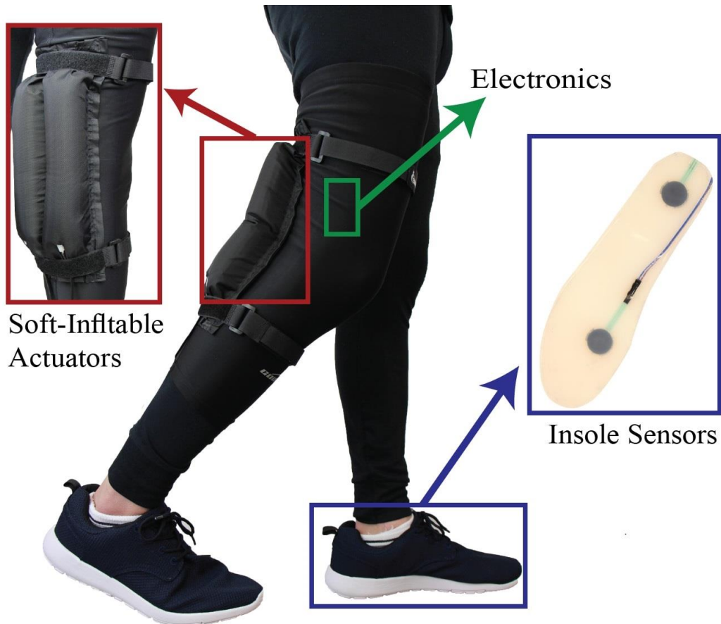
Figure 13. Components of the soft-robotic knee exosuit used for evaluation in stair ascent [28]
