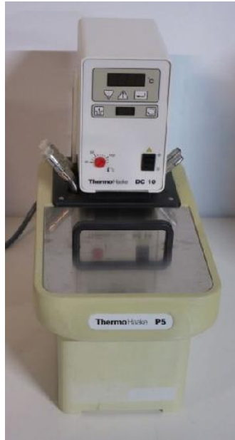
Fig 20: Thermostat used for calibrating the thermocouples.
