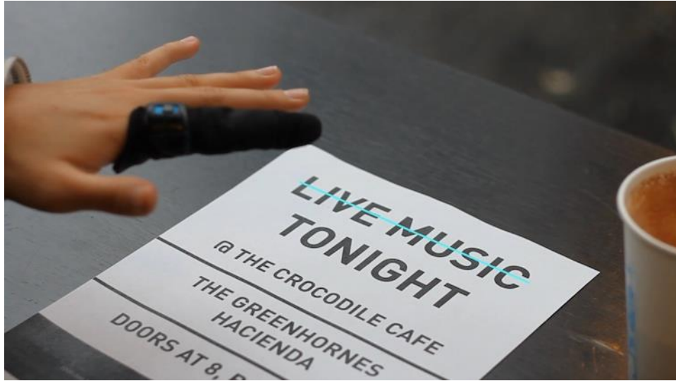
Figure 5: Electro tactile braille display
