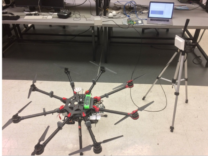
Figure 2.3: Electromagnetic micro-Doppler measurement experimental setup. A 100 kHz tone is transmitted at 5.8GHz with a sampling rate of 1MHz. Two 5.8GHz 11dBi flat patch antennas are used. Antenna height: 1.3m. Distance to drone: 1m. Angular separation: 15 degrees.
