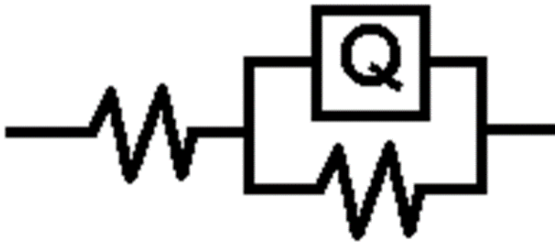
Figure 7: The above circuit is a modified randel's cell. Q, represents constant phase element which is has been commonly used to represent an imperfect capacitor. The two resistors represent the electron transfer, and solution resistance.
