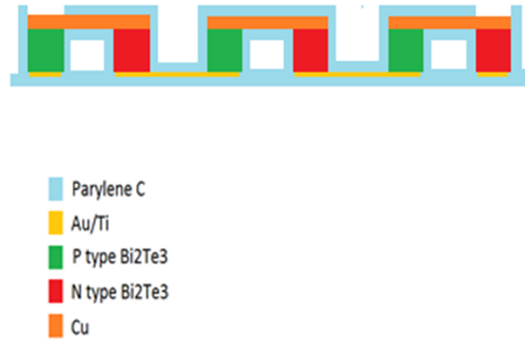
Figure 2.17 Device Structure of the Flexible Thermoelectric Generators
