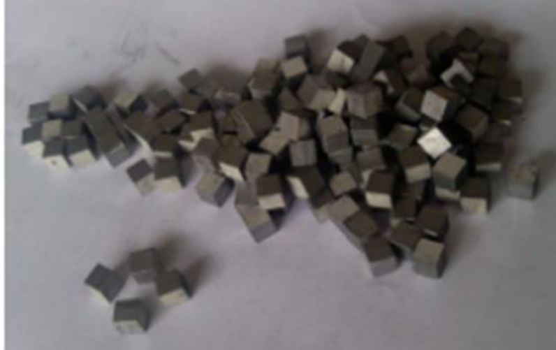
Figure 3.1 Bismuth Telluride Pellets (1.4x1.4x1.1mm) Purchased from Everredtronics
