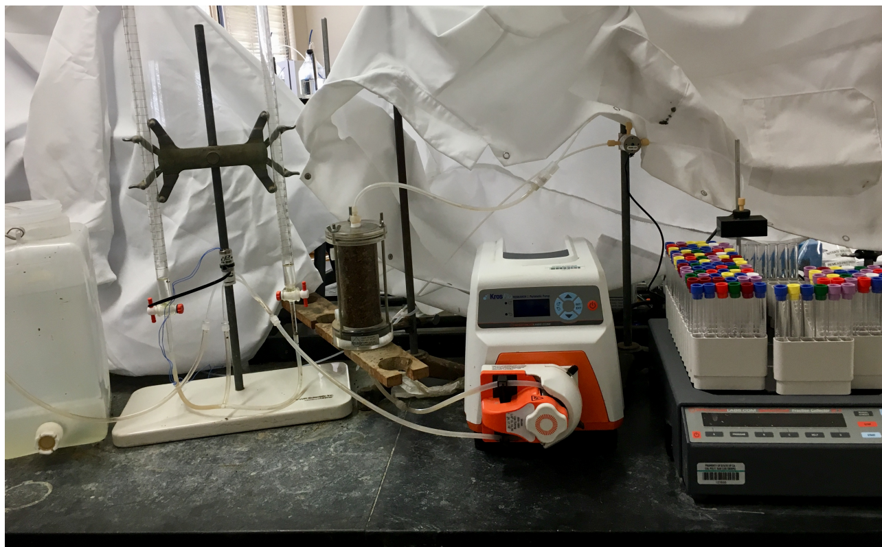
Figure 1: Experimental setup of breakthrough experiments, described from left to right: water container holding flush solution; two 100 mL burettes containing dilute \text{KNO}_3 solution; soil permeameter; KrosFlo peristaltic pump; fraction collector with test tubes.
