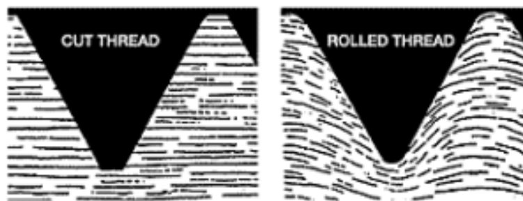
Figure 3. A representation of the difference between thread cutting and thread rolling. Thread rolling deforms the grains, increasing the strength of the threads [5].
