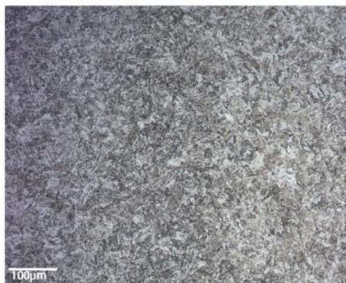
Figure 6. Microstructure visible under optical microscopy, showing martensitic matrix [1].
