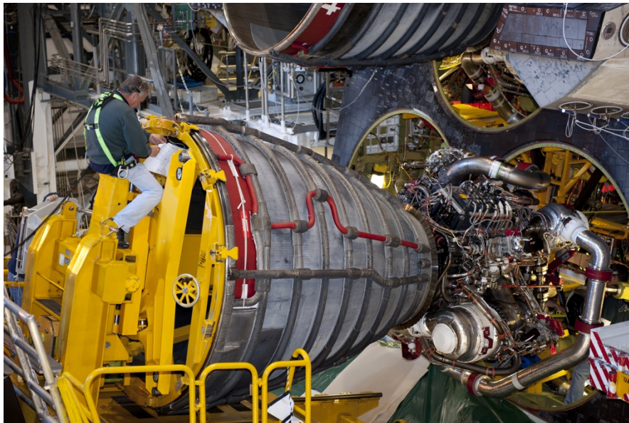
Figure 1. A field engineer guiding the installation of a RS-25 engine. 2
