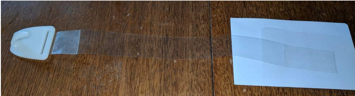
Figure 8. Commercial GripHanger™. One-inch by 2-inch surface-area polymer pad on right, attached to packaging to preserve surface to be stuck to glass and placed on top of an index card for visibility.
