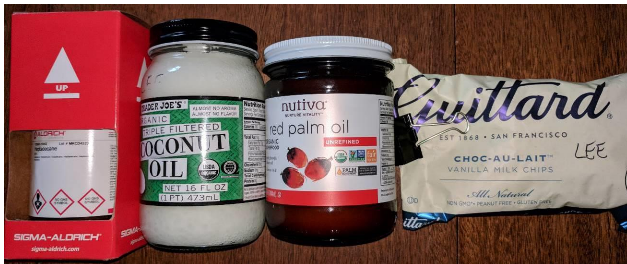
Figure 2. Candidate PCM materials. From left to right: Heptadecane, coconut oil, red palm oil, and white chocolate.
