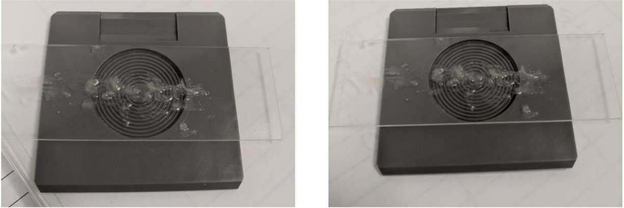
Figure 16. Photos of calcium chloride salt before and after X-ray irradiation. No significant color change was observed.
