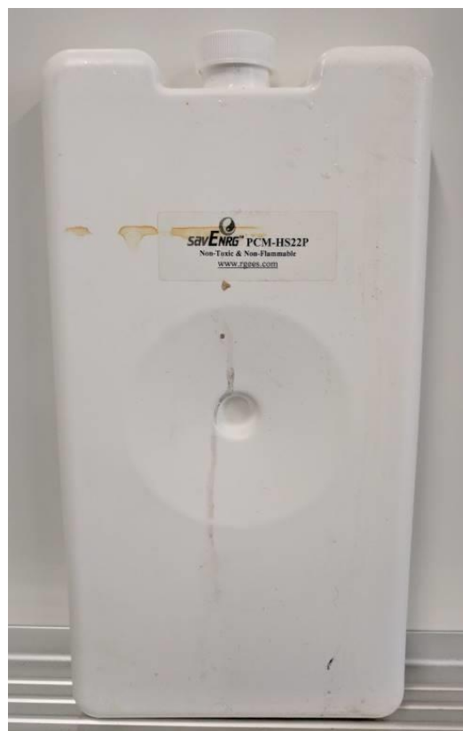
Figure 4. Container of technical palm oil manufactured by SavEnrg. Waxy and opaque when solid; clear when liquid.
