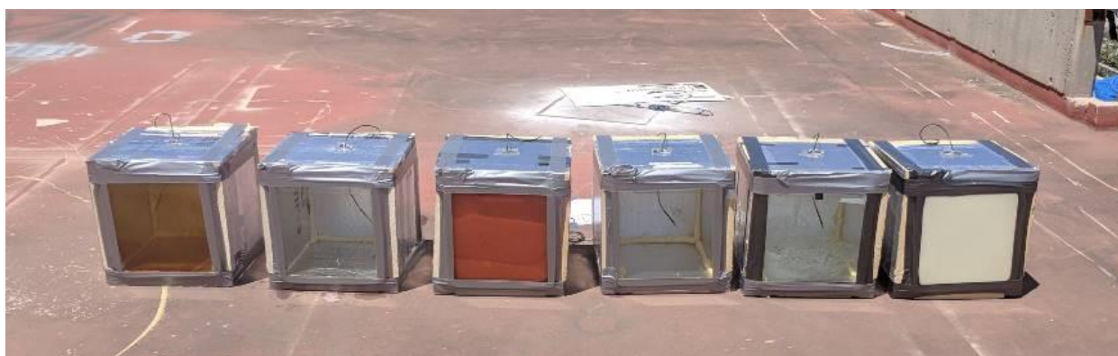
Figure 13. Proof of concept experiment setup. From left to right: Tiles filled with honey, coconut oil, red palm oil, heptadecane, PureTemp's palm oil, and white chocolate.
