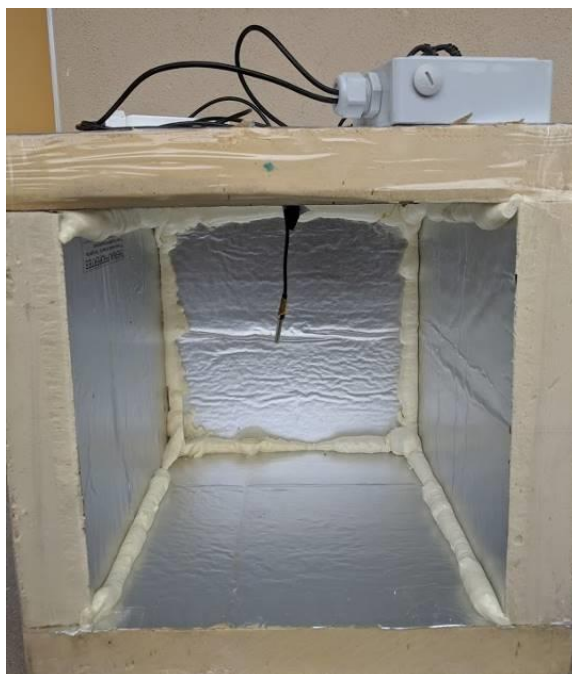
Figure 12. Interior of proof-of-concept experiment box, showing insulating foam and HOBO temperature probe at top.
