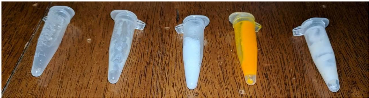
Figure 6. Candidate PCMs prepared in 2 mL vials for the melting temperature measurement. From left to right: Heptadecane, calcium chloride salt, coconut oil, red palm oil, and white chocolate.
