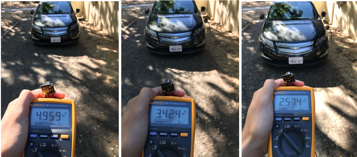
Figure 17: Readings for Analog Voltage Output from Sensor
