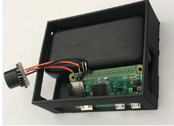
Figure 16: First 3D Printed Encasement
