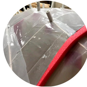
SPILL EDGES ARE DEFINED USING POLYURETHANE TUBING AND PVC PIPES
