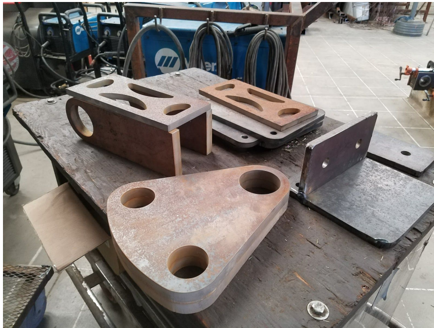
Figure 62. Completed water jet plates
