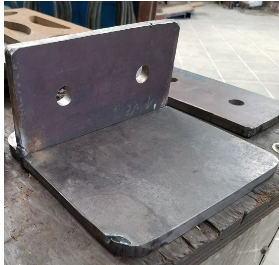
Figure 66. Back cylinder mount tack welded for marking holes
