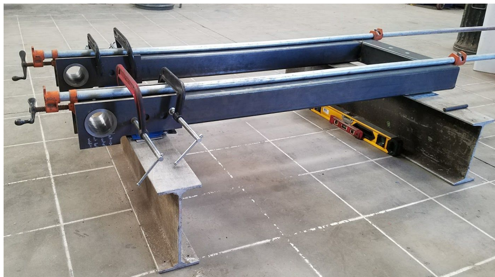
Figure 67. Leveled assembly for marking holes
