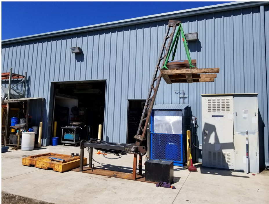
Testing at 1500 lbs with 10 ft truss.
