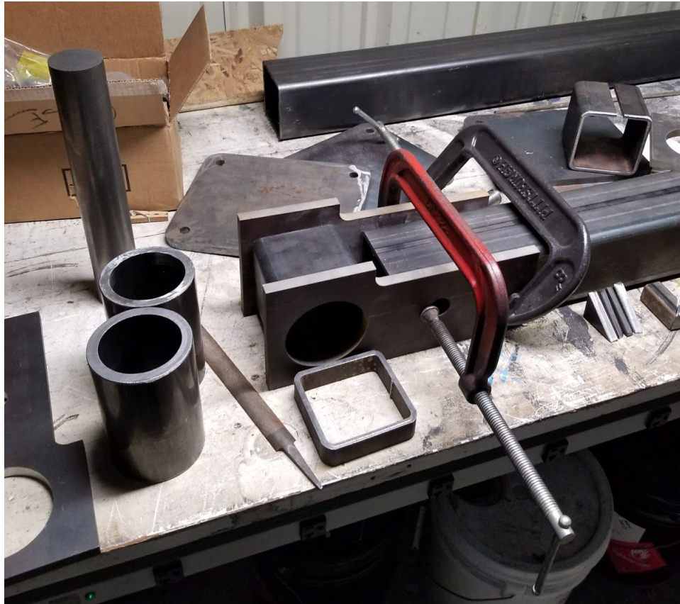
Figure 63. Box steel and pipe sleeve manufactured for shaft assembly
