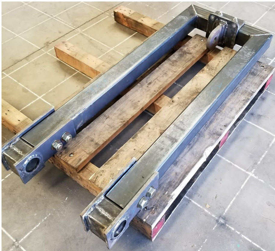
Figure 68. Fully welded shaft and base frame assemblies
