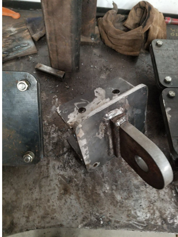
Rear Cylinder mount, must be removed completely to remove cylinder
