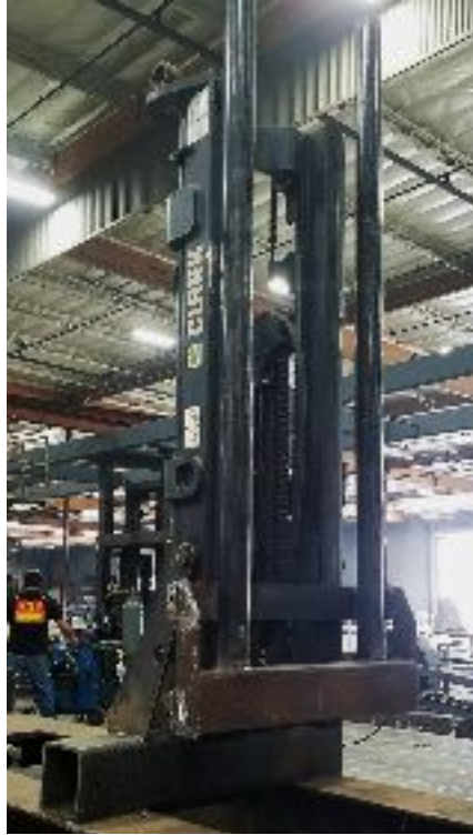
Figure 14. Overheight Mechanism Using Forklift Mast
