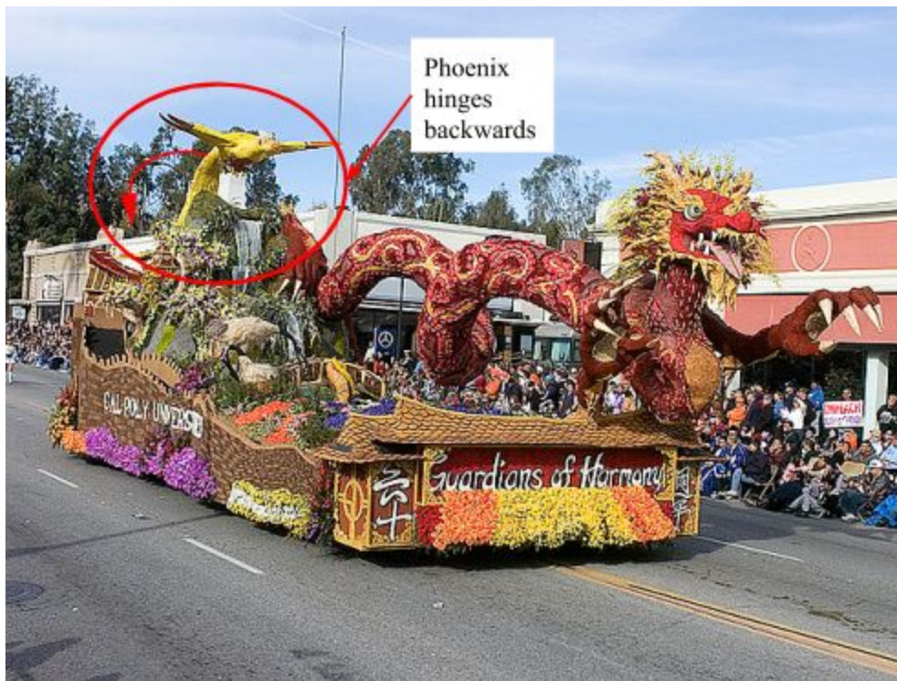
Figure 10. Cal Poly's Guardians of Harmony Float with Hinge Mechanism
