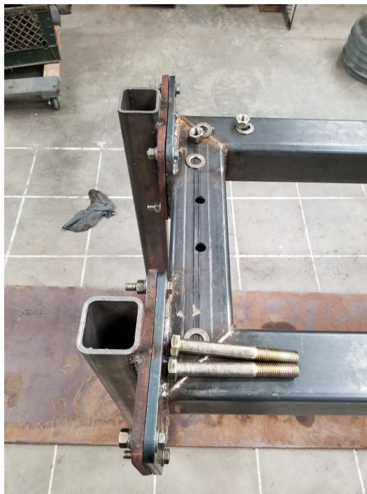
Back side of mechanism, showing back mounting location and two rear match plate locations
