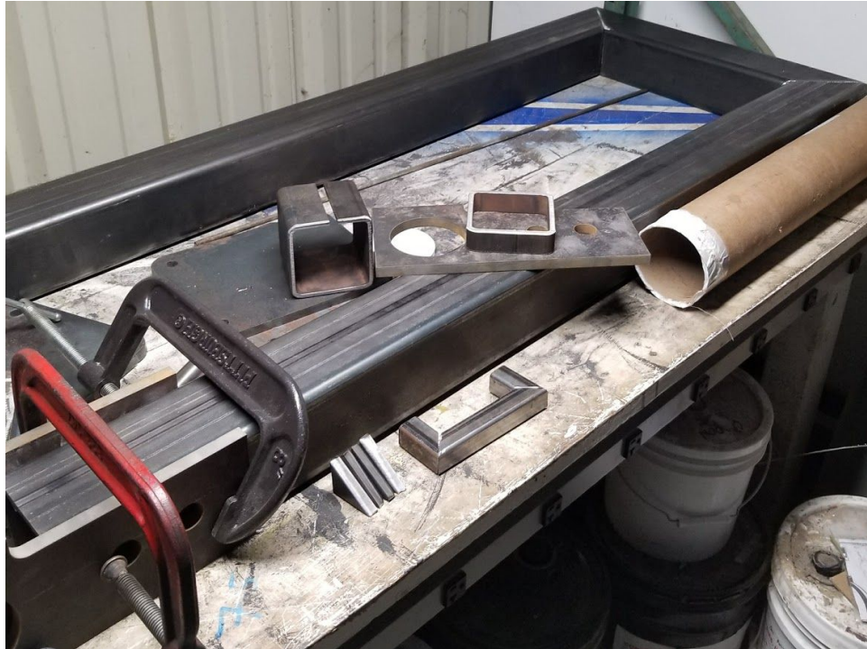
Figure 60. Box steel cut for frame and shaft sub assembly
