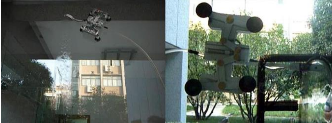
Figure 13: Linkage driven pneumatic climber [14]
