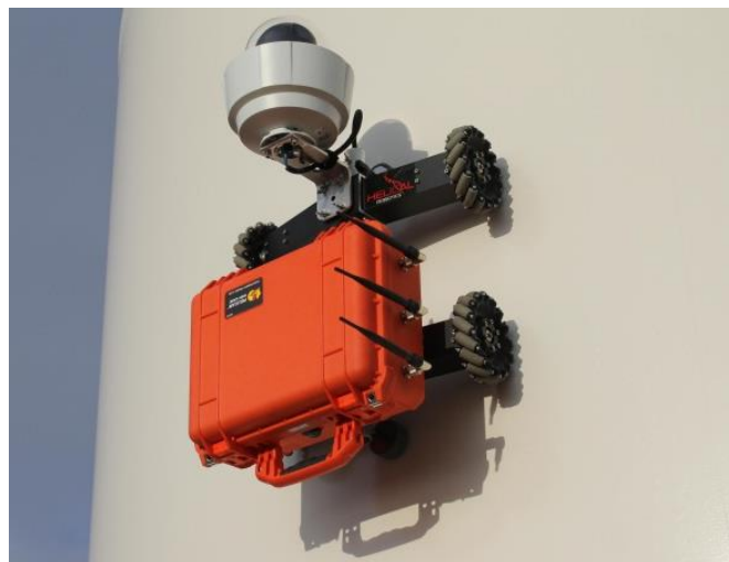
Figure 4: A magnetic wheeled robot [4]
