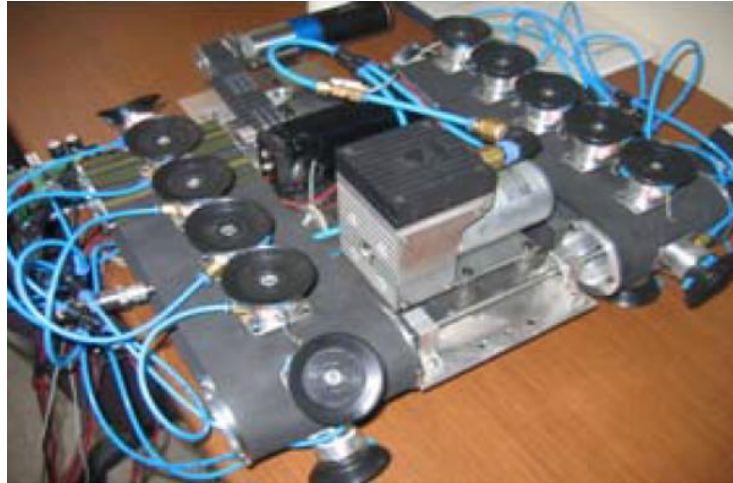
Figure 8: Treaded active pneumatic vehicle [8]
