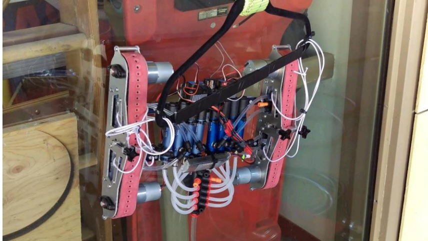
Figure 67: Video frame, vertical climb on glass
