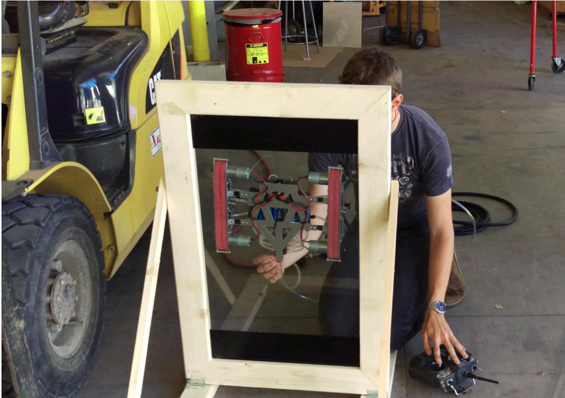
Figure 59: Still from video showing the first successful climbing test on adjustable glass surface
