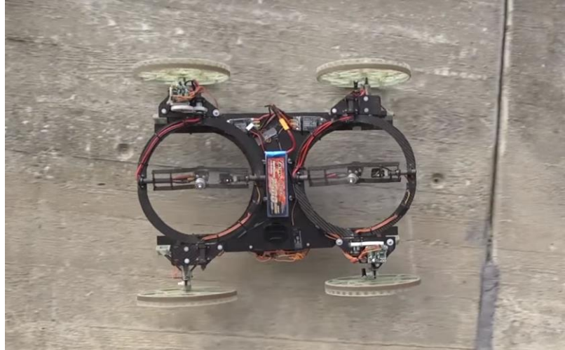
Figure 3: TheVertiGo, a wheeled robot using directed thrust [3]
