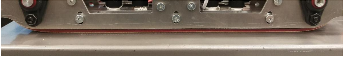
Figure 64: Manifold height properly adjusted, creating flush sealing surface
