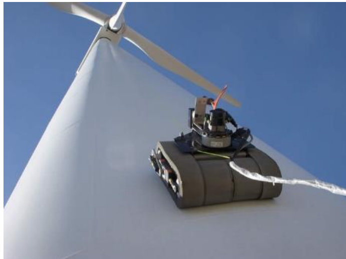
Figure 9: Treaded vehicle with central active pneumatic system [9]
