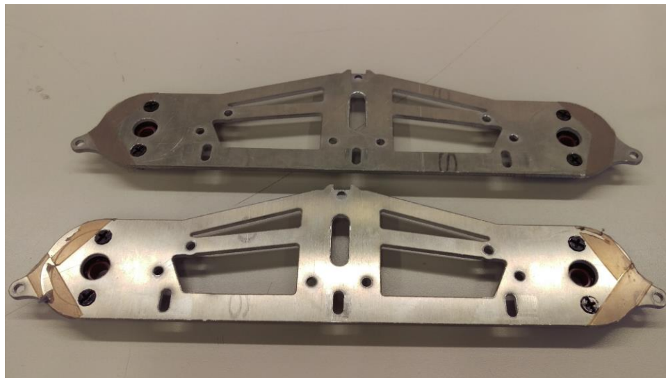
Figure 65: Damaged PTFE tape due to loose drive pulley set screws
