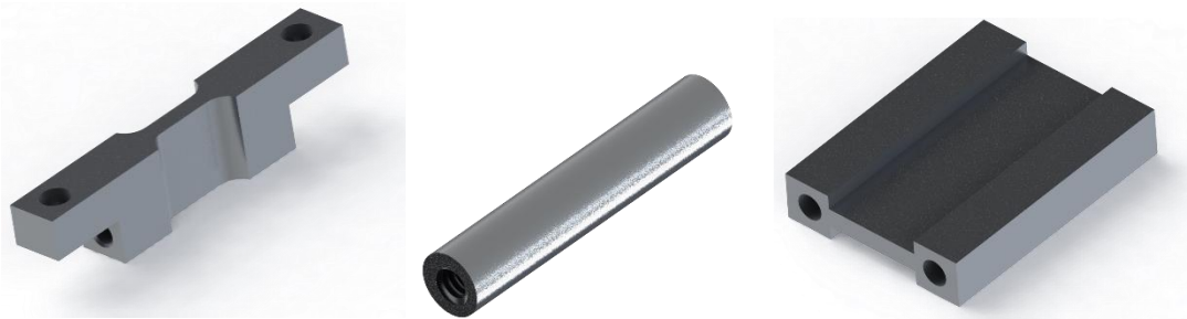
Figure 39: Renders of the secondary machined components
