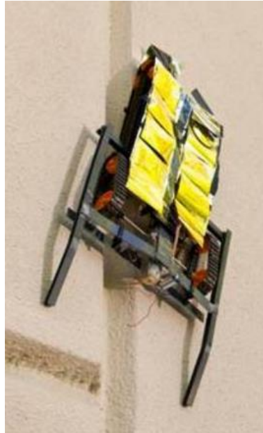
Figure 10: Small vehicle based on electrostatic adhesion [10]
