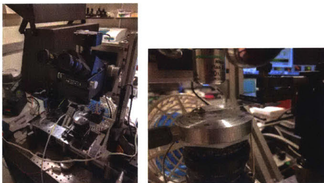
Figure A-3: Photographs of the home-built transfer setup used to move 2D materials between various substrates. The close up image on the right shows a heated XYZ stage, with vacuum chuck, and a cantilevered glass slide on a XYZ manipulator.
