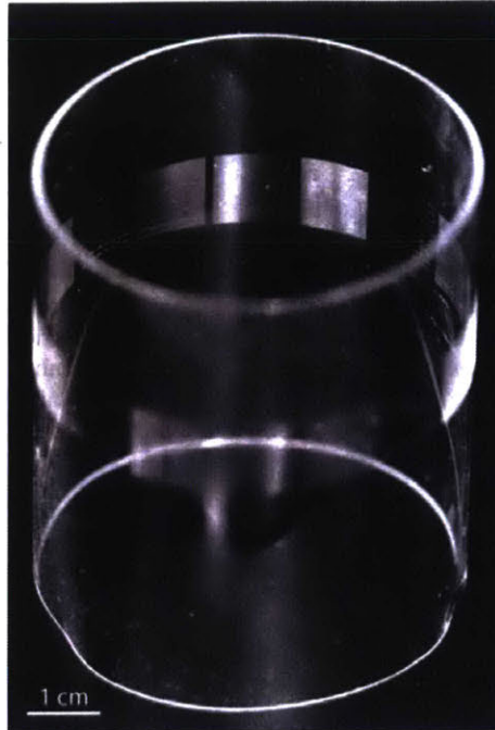
Figure 1-8: Seamless cylindrical stamp . A finished seamless cylindrical stamp. This stamp, produced by Ascoli, had a set of discontinuous patterns to investigate stamp production capability. [22]
