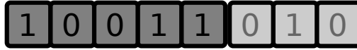
FIGURE 3.3: A simple 1-byte example representation of an antigen (in the model four bytes are used). All 8 bits are used to encode the antigen's genotype, while only 5 bits contribute to the antigen type (shown in darker gray). There are therefore multiple possible genotypes for each antigen type.
