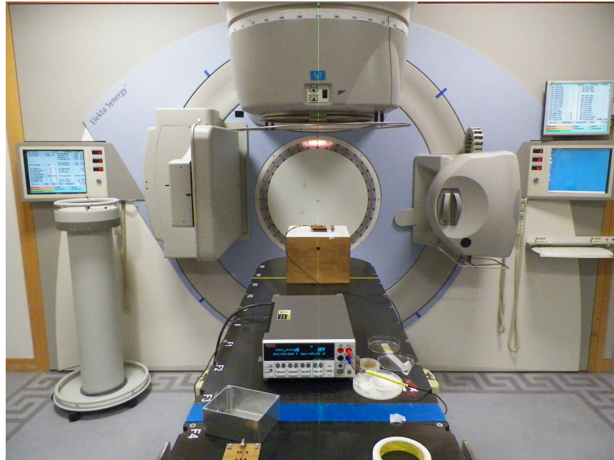
Figure 1.5: A stereotactic radiotherapy machine used at the Christie hospital in Manchester, with a diamond sample ready for testing.
