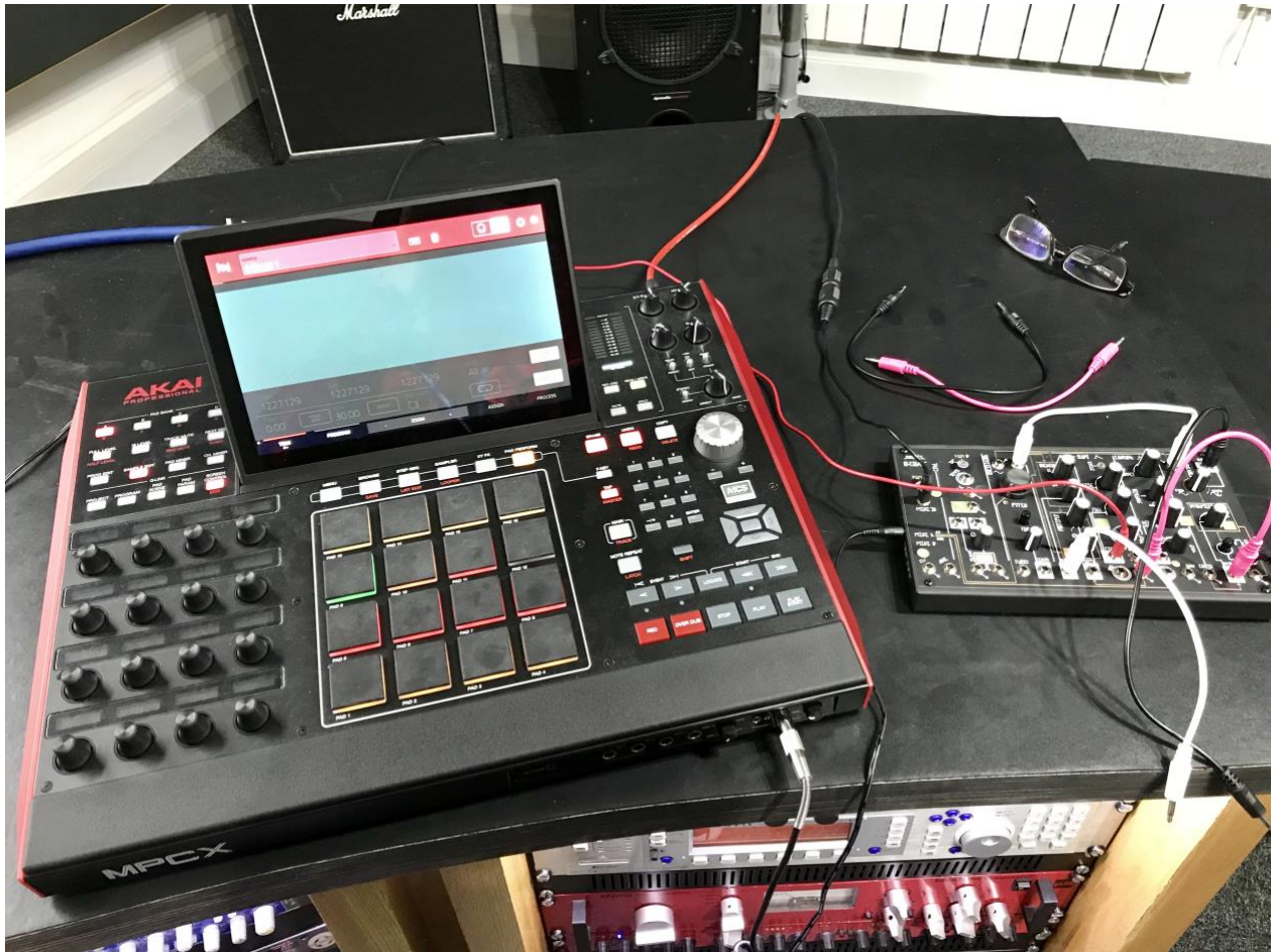
FIGURE 5. AN AKAI MPC X SAMPLER/DRUM MACHINE AND MAKE NOISE 0-COAST SEMI-MODULAR SYNTHESISER USED FOR SAMPLING, DRUM-PROGRAMMING AND SYNTHESIS FOR THE HIP-HOP/ELECTRONICA CASE STUDY.
