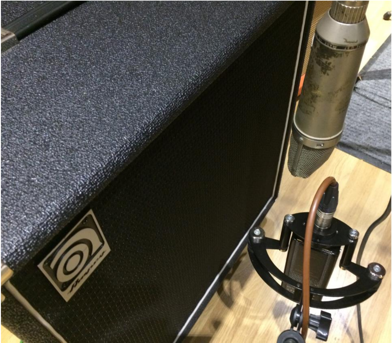
FIGURE 3. NEUMANN U 67 AND SONTRONICS SIGMA RIBBON MICROPHONES POSITIONED IN FRONT OF AN AMPEG BA-115 BASS AMPLIFIER WITH A SINGLE CELESTION SPEAKER.
