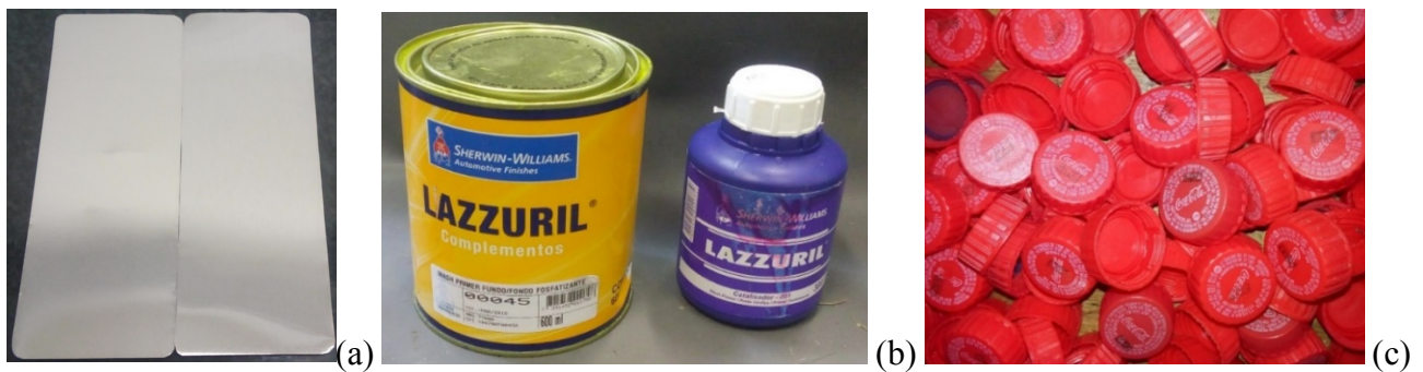
Figure 2. Aluminium skins (a), Wash Primer components (b) and disposed bottle caps (c) used for sandwich panel manufacturing.
