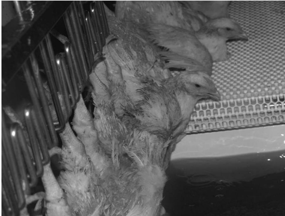
Figure 3. Breast support conveyor installed to support the weight of birds while they are shackled and inverted (Adapted from Lines et al., 2012)
