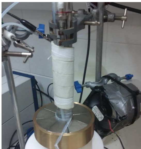
Fig. 4: Apparatus employed for initial trials on Eurofer-97 corrosion within a magnetic field.
