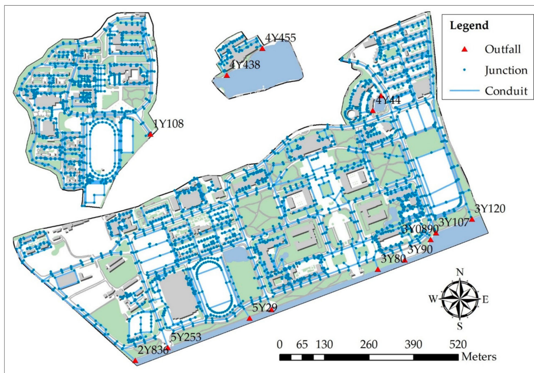
Figure 7. Distribution of the storm sewer networks in the three sub-basins. The red triangles represent outfalls, which are terminal nodes of the drainage system. The blue dots represent junctions where links join together. The light blue line represents conduits that move water from one node to another.
