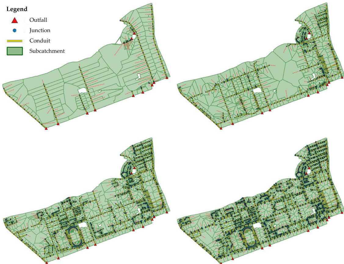
Figure 10. Classification results for four levels of the sewer network and the corresponding discretization results for the main district.
