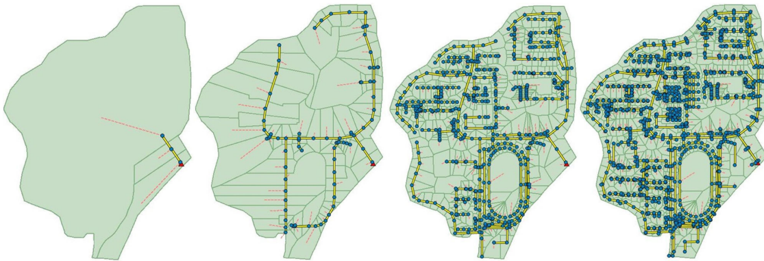
Figure 8. Classification results for four levels of the sewer network and the corresponding discretization results for the northern district.
