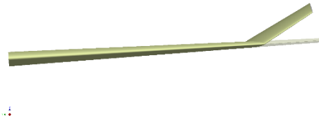
Figure 4: Front view showing positive fold angle for a hinge angle of 30^{\circ} .
