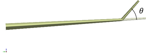
Figure 2 Fold angle \theta .
