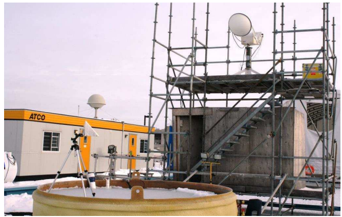
Fig. 1. Scatterometer measures the normalized radar cross section (NRCS) of the oil-contaminated sea ice. In this figure, an external calibration is being performed utilizing a metallic trihedral.
