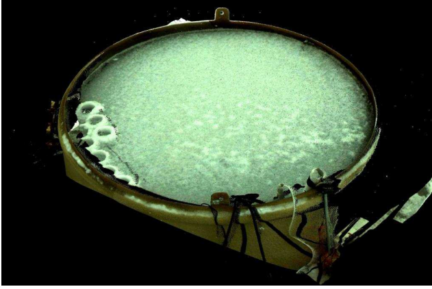
Fig. 2. A lidar scan of the profile's topography.
