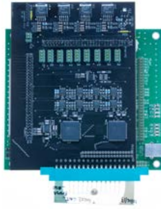
(b) Picture of the Mecobo motherboard with mixed signal daughter board.
