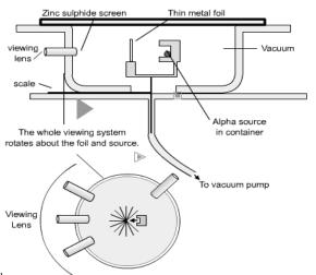
[Fig: Experimental setup for Rutherford's Experiment Image Source [1]]
