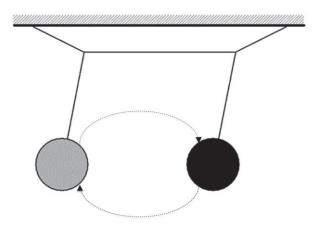
**Figure 2.** Two oscillating (i.e. coupled random dynamical) systems, A and B, suspended from a beam that is itself able to move. The two arrows illustrate the coupling between pendulum A and pendulum B (for additional discussion, see [16]).
