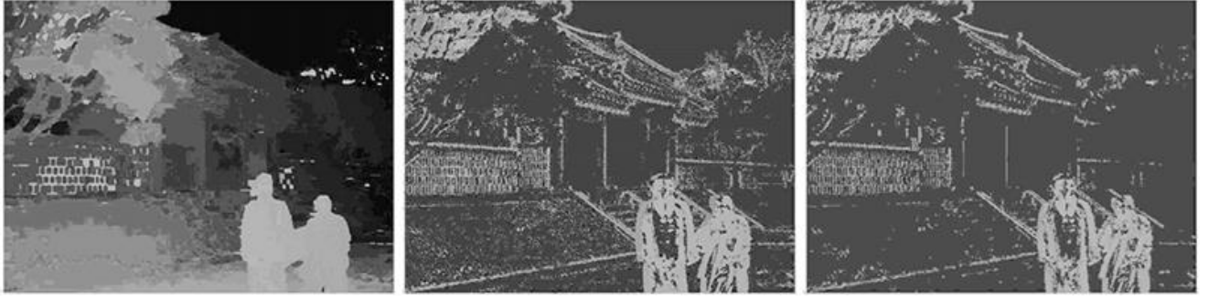
Fig. 3. Disparity maps and filtered disparity maps of Love Bird (CB = 100 mm and p = 8\% ). From left to right: disparity maps, filtered maps by (4), and filtered maps by color difference maps by (5). We enhance these images using histogram equalization for better visualization.
