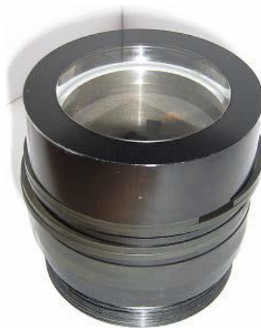
Figure 3.2. Optical flat piston with quartz piston-crown
