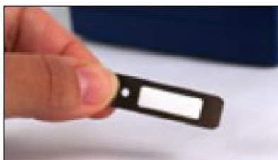
Metal side of filter strip faces bottom.
