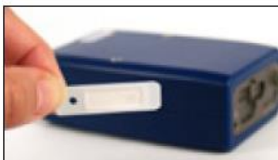
White side of filter strip is sample deposit side. White side faces up.
