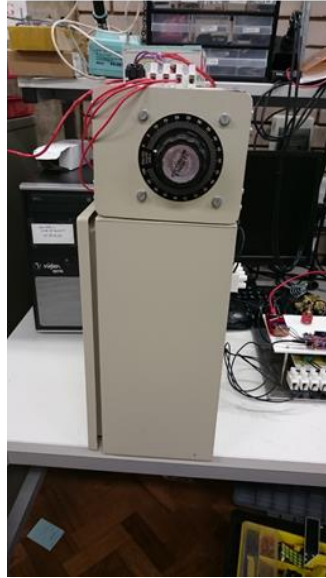
Figure 60 The Variac Transformer used for this study.
