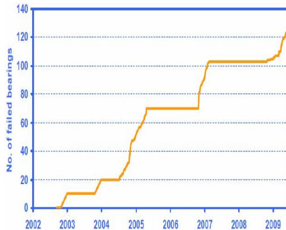
Figure 33 Planetary bearing failures at Horns Rev 1 offshore wind farm reported by Vattenfall [96]
