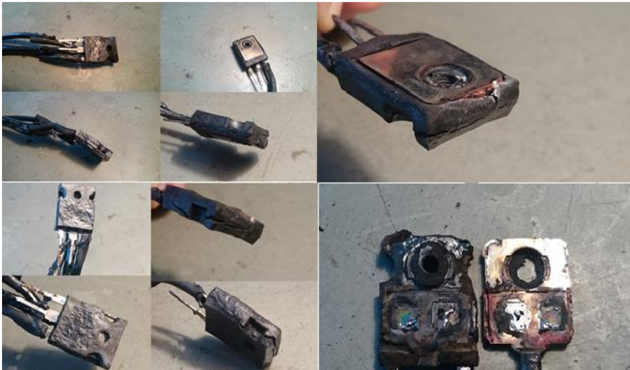
Figure 67 Failed IGBTs retrieved at the end of simulations.
