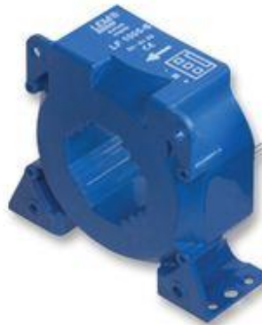
Figure 95 Photograph of LEM LF 305-S. The photograph is courtesy of INDRA.
