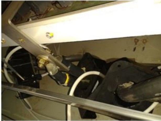
Figure 104 Inverter current sensor. The photograph is courtesy of INDRA.
