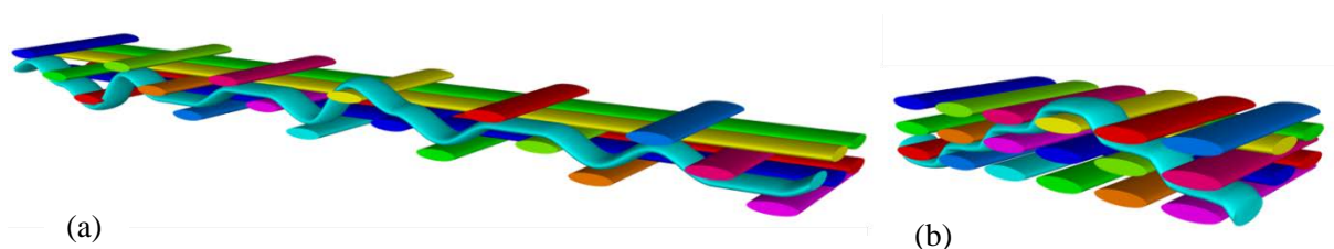
Figure 9. Angle interlock textile a) unconsolidated b) after consolidation
