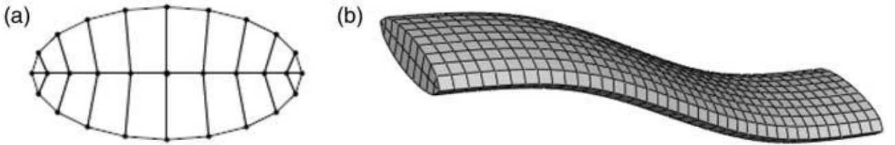
Figure 5: Conformal mesh generation, (a) 2D section mesh, (b) 2D meshes joined to form hexahedral and wedge elements
